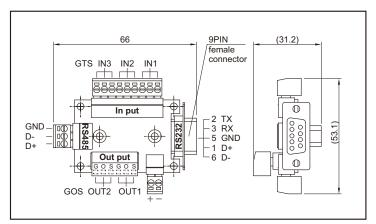
When in control mode, all inputs/outputs are not defined and should be defined by program. (I/O card is optional)
